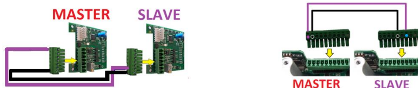
Fig. 12 – MASTER/SLAVE anslutning 0-10V
