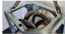
Fitting lifting lugs in the positions provided
